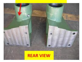
Brackets with counter bore grease fitting holes. One front and one back
